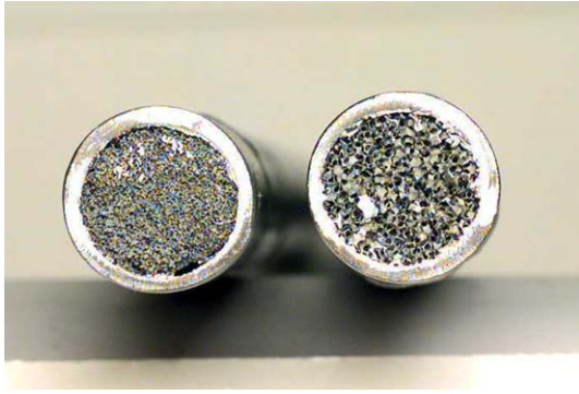
Fig. 1. Metal-foam filled tubes using co-sintering technique.
